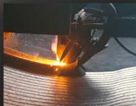
Pressure Vessel Cladding
